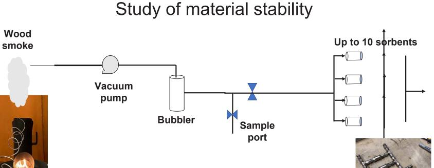
Expose materials to exhaust of biomass combustion (i.e., wood burning) for 6 hours and test material properties before and after exposure
