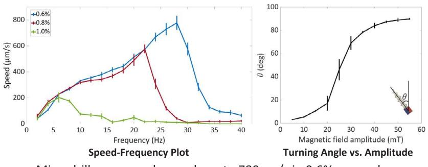
• Microdriller can reach speeds up to 780µm/s in 0.6% agar gel
